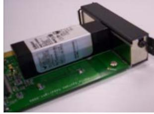
**Note:** You must attach the bracket to the PCI adapter card before you slide it into the PCI slot.
