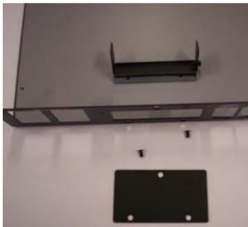
5. Unscrew the screw in the bracket. The 8-port/16-port/32-port bracket is shown below.
