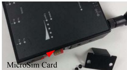
1. Removed the screws from the side of the SDS L unit, then remove the cover plate.
